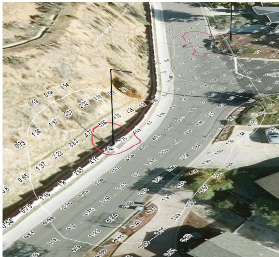
Horizontal illuminance calculated on actual terrain in GIS. The slope, curve, and pole position are unique to this location. A typical layout on a flat surface would produce different results.
