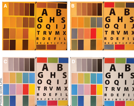
Color chart illuminated by a) HPS, b) 1800K LED, c) 2200K LED, and d) 2700K LED luminaires. Individual color panels were visually distinct and identifiable under all LED spectra.
