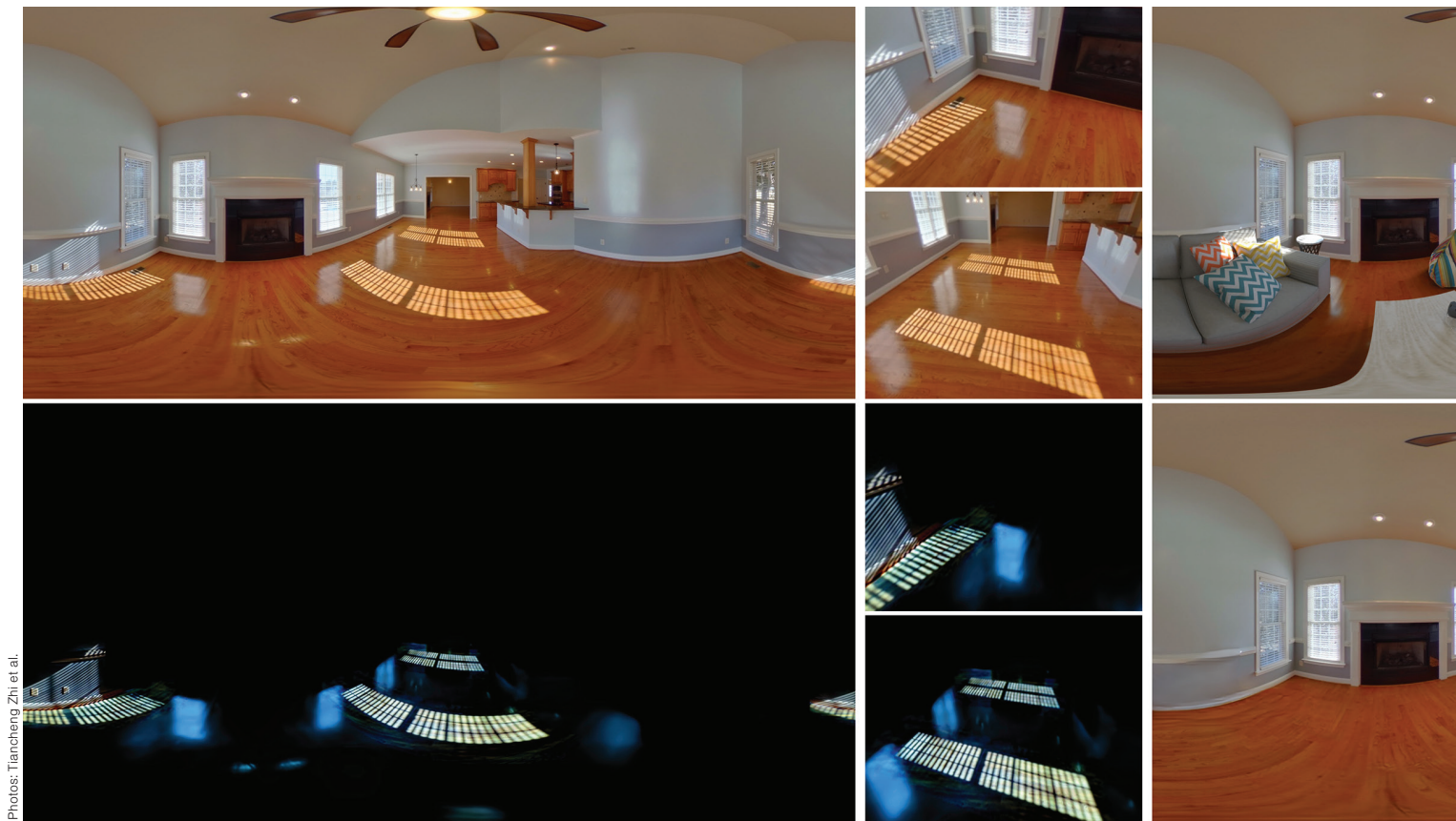
Figure 3. An example of a single panorama of an empty indoor scene (top left) is decomposed into appearance components on the floor and walls: specular and direct sunlight (bottom left) and diffuse ambient light without direct sunlight (bottom right). Then, the scene is virtually staged with new furniture insertion (top right).
