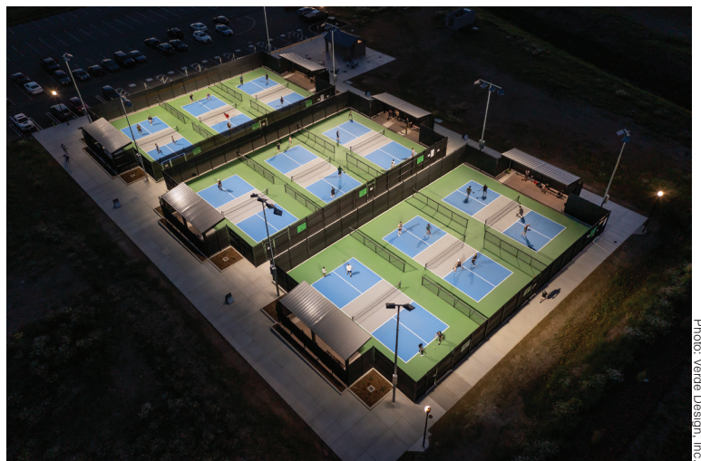
The Courts at Gibson Park, a pickleball complex in Roseville, CA, features eight 580-W fixtures per court with an average of 45 fc.
