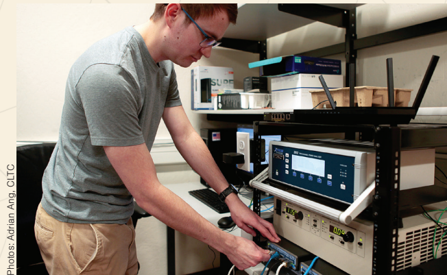
A CLTC engineer connecting a network traffic generator to the networking equipment testbed.
